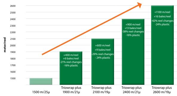
Based on: Round bale 1,20 m, 6 layers of film, 55 % overlap, 70 % pre stretch, when comparing to 1500 m/25µ film.
